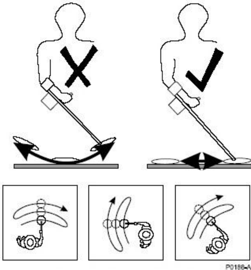
Figure 18 - Sweeping the Coil
